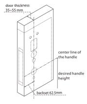
Note 1: Align the template along the vertical center line of the mortise (E) at the desired handle height, and tape it to door.
