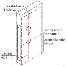
Note 1: Align the template along the vertical center line of the mortise (F) at the desired handle height, and tape it to door.
