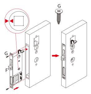
Note: Ensure the two triangles are in horizontal alignment.
