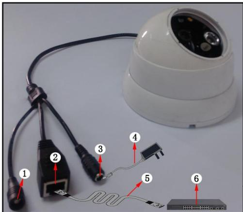
I . Connect the power cables and power on the MD532.
