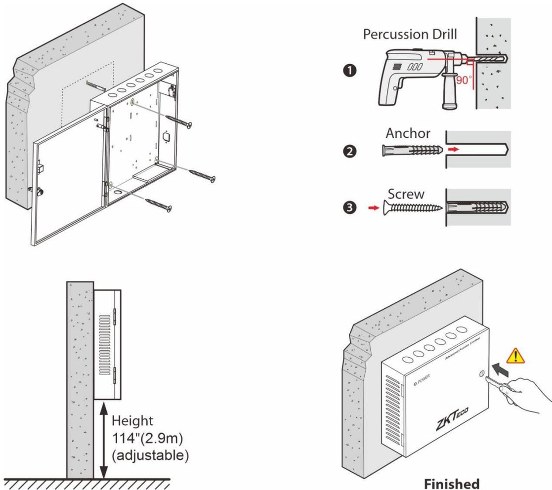
**Figure 3-1** Installation the metal enclosure on the wall
