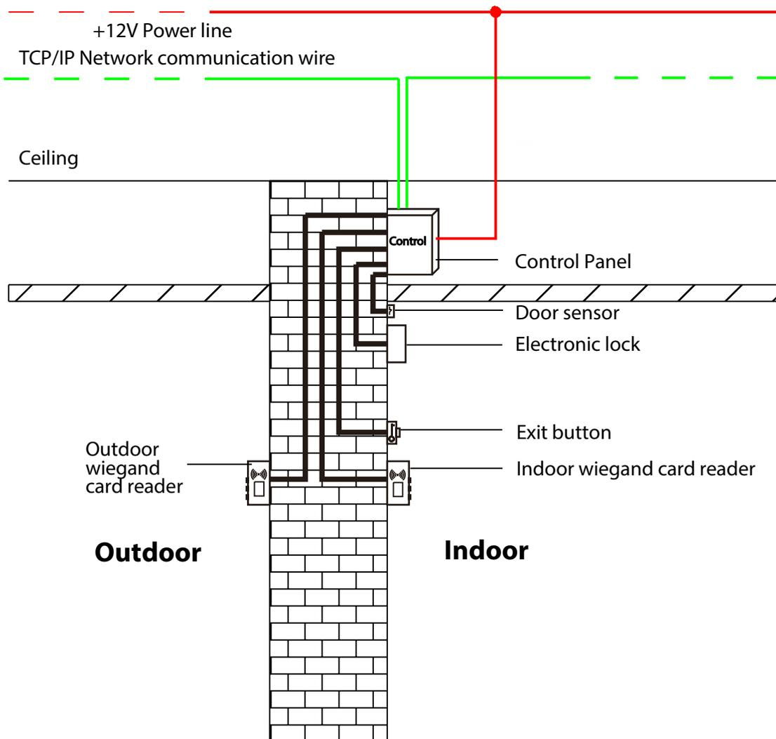
**Figure 3-2** Access Control Panel Wire Installation Diagram
