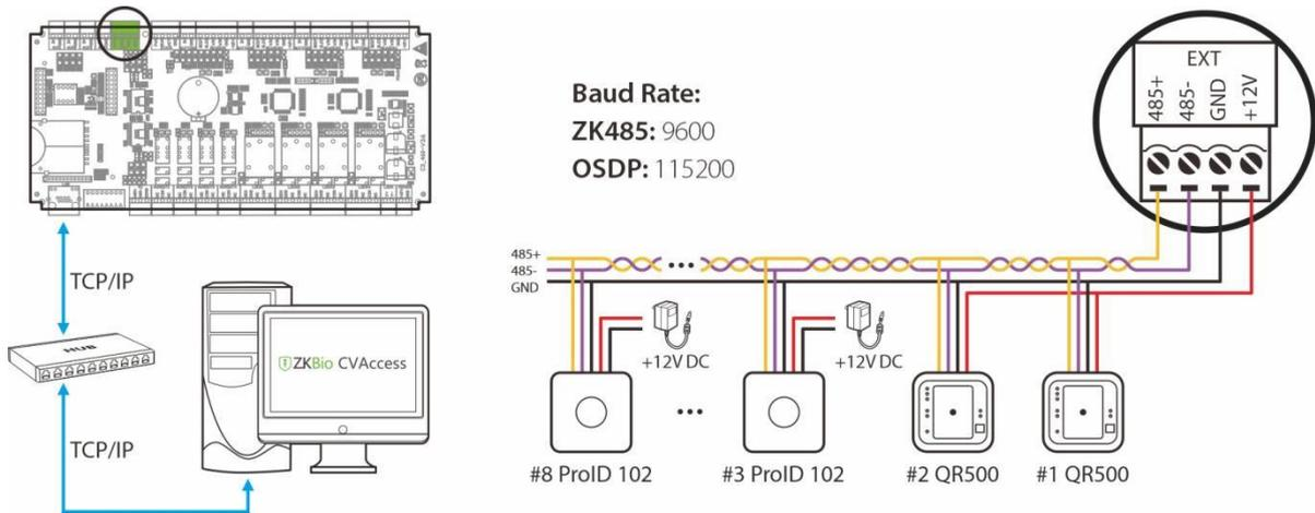
**Figure 4-10** Connection between C3-400 Pro Plus and RS485 Readers
