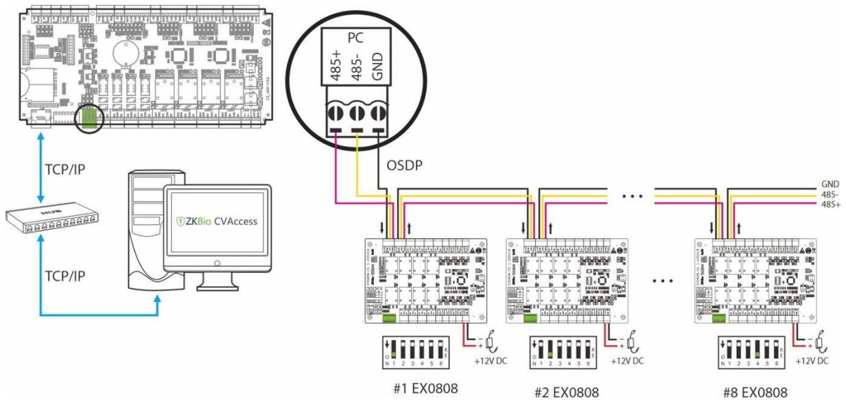
**Figure 4-12** Connecting the EX0808 expansion board via PC485
