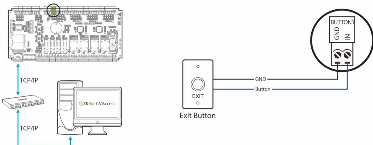
**Figure 4-9** Exit button supply wiring diagram
