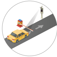
LPR Camera scan the number on the license plate when vehicle is approaching its reading range
