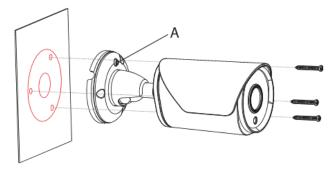
3. Three-axis brackets adjustment: loosen the camera body's screws to adjust the three-axis. Adjust the connection between brackets and basement by axis to implement 0°~360° in the horizontal direction. Adjust the spherical joint of brackets to achieve 0°~90° in the vertical direction and 0°~360° in the rotational direction. Tighten the screws after adjusting the desired camera position. Installation is then completed.
