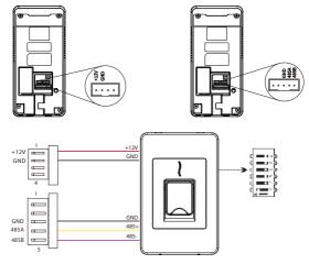
When using the reader with Standalone access controller device, please move the dial code "1" to the ON position as shown above.
