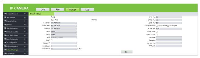
**LAN:** Set the related parameters of a Local Area Network, including IP Address, Subnet Mask, Gateway, DNS and MAC according to the actual situation, click [Save].
