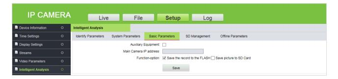
**Auxiliary Equipment:** The master-auxiliary mode recognizes the license plate and sends the recognition result to the main camera. Please select the Auxiliary Equipment check box if you want to use this feature.
