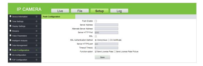
**Push Enable:** Select the check box to enable this feature.
