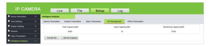
When the camera uses the SD card, this page shows the total capacity, used capacity and remaining capacity of the SD card. You can format and re-use the SD card.
