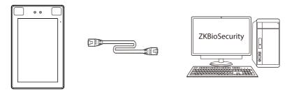
Default IP address: 192.168.1.201 Subnet mask: 255.255.255.0 IP address: 192.168.1.130 Subnet mask: 255.255.255.0
