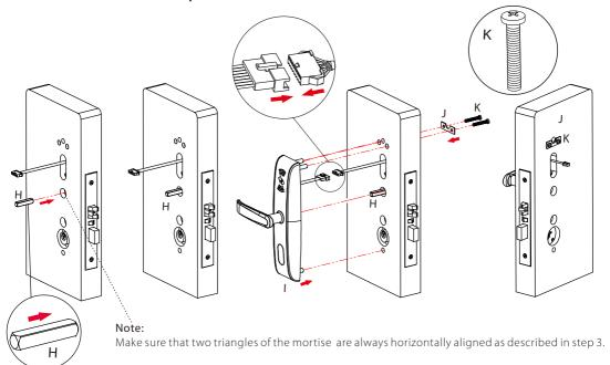
7. Attach the 8x8 spindle (H) and 5x5 spindle (L). Then fix the
