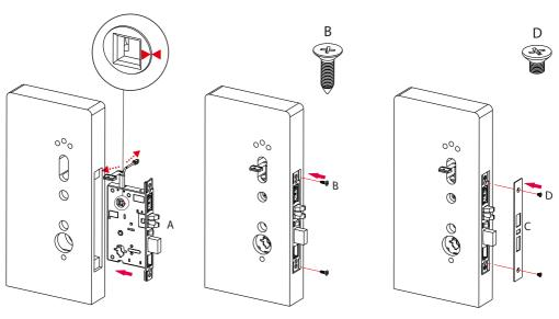
**Note:** Two Triangles on the mortise must be aligned horizontally (as shown in the above image).
