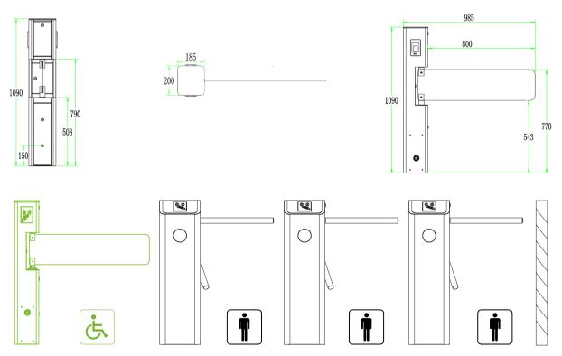
SBT1000S is usually used with other types of turnstiles together. It is suitable for trolleys, wheelchair passthrough, and is not suitable for high-traffic volume.
