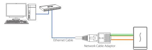
2) The device directly connects to the computer.
