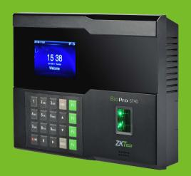
BioPro ST40 & ST40-A is a fingerprint identification time & attendance and access control terminal, which can connect with third party electric lock, door sensor and exit button etc.
