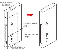
**Note1:** Align the template along the vertical center line of the mortise(E) at the desired handle height, and tape it to door.
