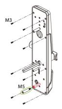
**Step 1:** Twist down the eight M3 screws and M5 stud bolt to take down the mounting plate.
