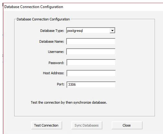
2. You need to select correct database and enter the correct parameters. Then click *Test Connection*. It will display "Database connection successful" if the connection was successfully made.
