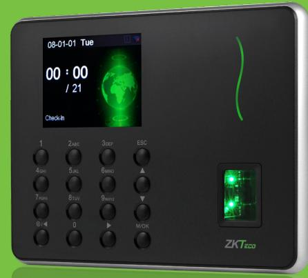
WL10 is Fingerprint Time & Attendance Terminal with Wi-Fi module. With Wi-Fi function, User needn't wire Ethernet cable, It's associated with ZK new fingerprint reader, the operation remains stable under strong light source and high precision of verification of wet and rough fingers. It also has elegant design and slim sharp, it will start new stage of time attendance.
