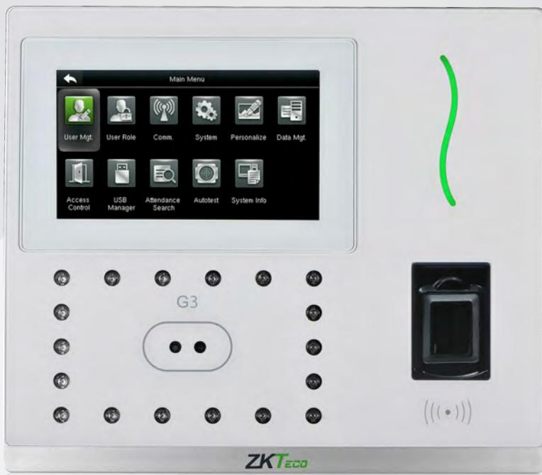
**G3** is a multi-biometric identification terminal which features ZKTeco's innovation Silk ID fingerprint sensor technology. With the world's cutting-edge 3D Neuron Fingerprint Algorithm, it precisely authenticates dry, wet, or rough fingerprints efficiently and accurately. Infrared technology enables the device to function automatically when fingerprints are detected. With the latest facial algorithm, it supports fake face detection.
