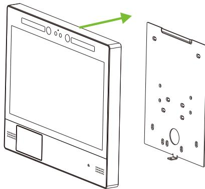
5 Secure the Kiosk by assembling the device and the rear panel with the bottom screws.
