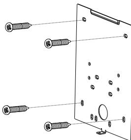
4 Set the device in an appropriate position on the rear panel that is fixed on the wall.
