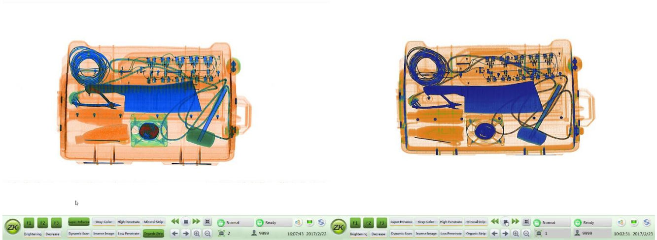
Figure 4 - Different colors of each materials (5030A right side)
